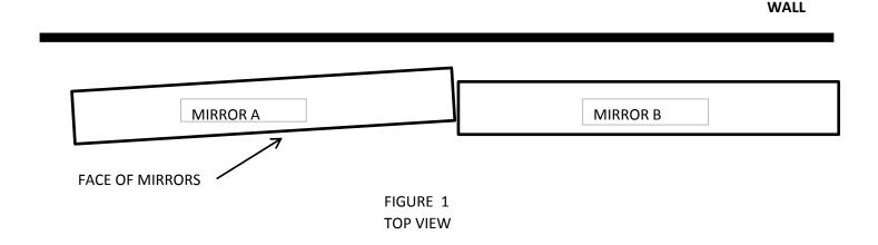
4) GENTLY PUSH BETWEEN THE WALL AND THE BACK OF THE MIRROR UNTIL FACE OF BOTH MIRRORS ARE EVEN--SEE FIGURE 2.
