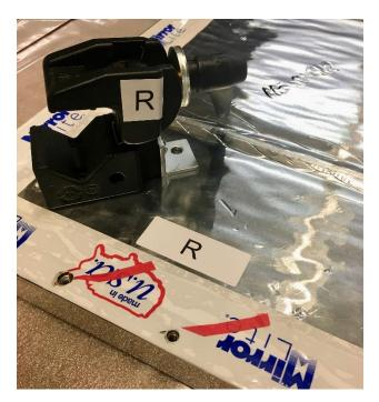
Step 6: Line up clamps Left or Right per label with one ¼-20 machine screws and one #10-24 screws into holes by red tape. Evenly screw down base of bracket.
