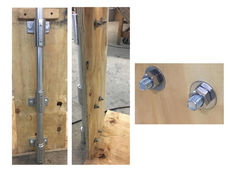
Step 2: Attach cross bars together. Unite cross bar A&B with cross bar A and then tighten fitting B with allen key provided. Remove blue labels after assembled.
