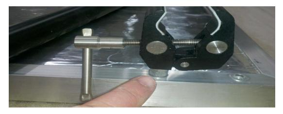
7) Lay cross bar into clamp jaws and gently tighten clamp. Do Not crush X-bar.
