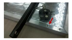
2) Line up ¼-20 machine studs into holes by red tape.
