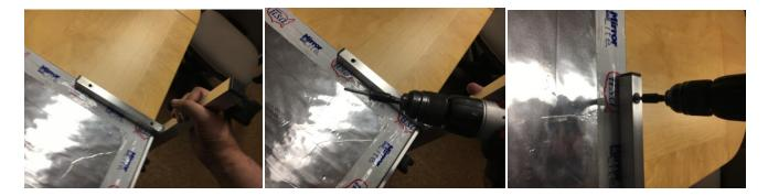
3) ONCE SCREW THREADS INTO ALUMINUM FRAME, REDUCE TORQUE ON DRIVER TO PREVENTSTRIPPING OF SCREWS. REPEAT STEPS FOR REMAINING SCREWS. SAVE HEX DRIVER FOR DISASSEMBLY IF STORED OR TRANSPORTED. REPEAT FOR OPPOSITE CORNER OF MIRROR.
